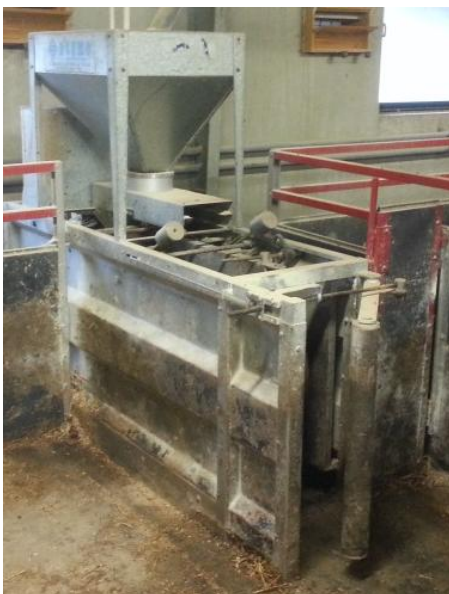
Figure 2: Data collection in the Bøgildgård grower/finisher section. A) The ACIMA-48 feeding station, used to record the amount of feed consumed by the individual pigs. B) The pig scale, used to manually weigh the individual pigs. The individual pigs were identified with RFID ear tags.
