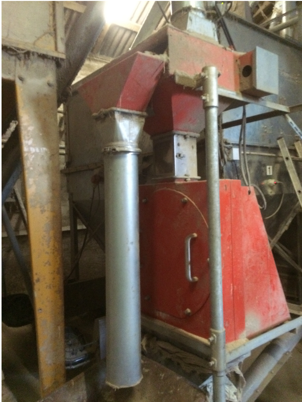
Figure 4.2: Combined grain cleaner and roller mill. Mixing vessel no.1 can be seen in the background.
